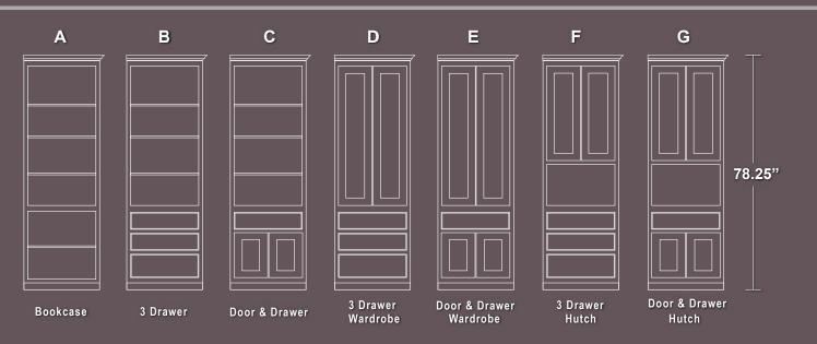
Width options for side cabinets: 18", 24", 30" Glass Door options for side cabinets: C - G Upper Door options for side cabinets: B - C Slide-out Night Tray options for side cabinets: A - G
